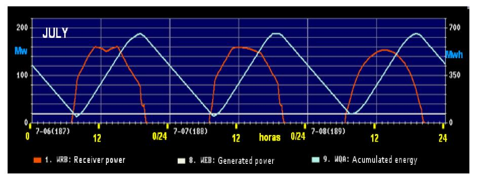
During the summertime, the plant supplies continuously energy to the grid
